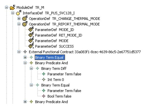
From this kind of model, the new version of the code generator can produce Ada 2012 specifications. As only the business code is concerned by Hi-Lite, the formal specifications are integrated in the code of the component implementation. For example:
